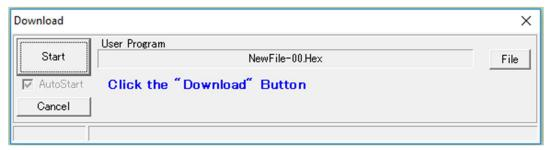
Downloading starts. On the robot, the LEDs should blink rapidly.
